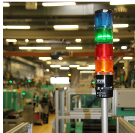
A signal tower fitted with the data collection transmitter on the production line in the Injection Moulding Department at Marquardt GmbH.
